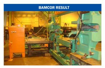
BAMCOR completes rebuild. Per our standard practice, temporary power is connected to the machinery at our facility for complete functional testing and sign-off prior to shipment.
