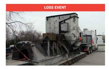
A new blower was built by the OEM and was crated at the loading dock for overseas shipment. The crate caught fire at the dock and heavily damaged the blower located within the crate.
